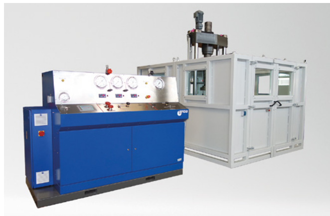
Figure 3: The vertical test bench PS-300 with automatic test sequence, slide-in carriage, proportional control and protective housing is suitable for shut-off valves with nominal diameters from DN 50 to 400.
